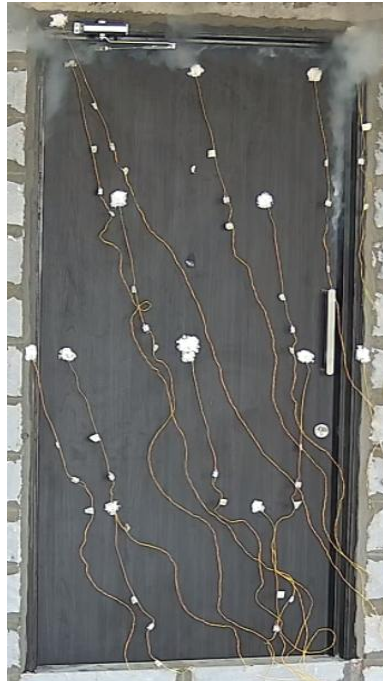
b) t = 05 min, grey smoke was observed emanating from the top edge of the leaf.
