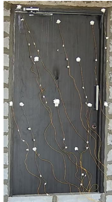
f) t = 60 min, increased blackening was observed near the door viewer.
