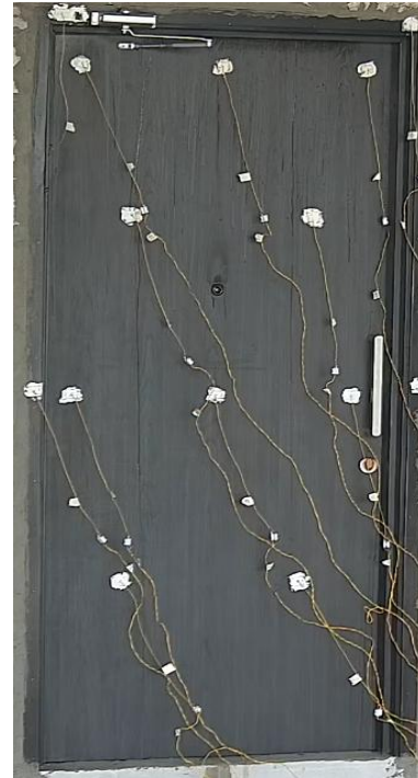
f) t= 60 min, oil leakage was observed from the door closer.
