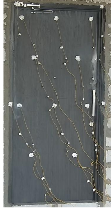
c) t= 15 min, heavy grey smoke emission was observed from the edges of the leaf.
