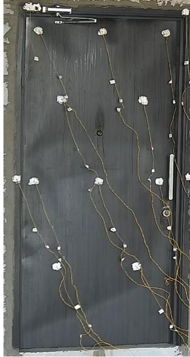
h) t = 90 min, formation of a bubble was noted on the door leaf.
