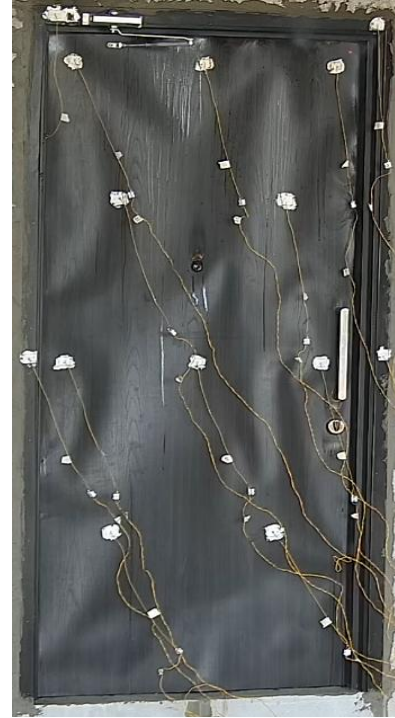
i) t = 105 min, complete swelling of the outer sheet of the door leaf was noted.
