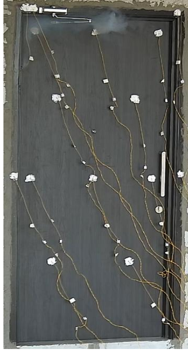
b) t= 01 min, grey smoke was observed emanating from the top edge of the leaf.
