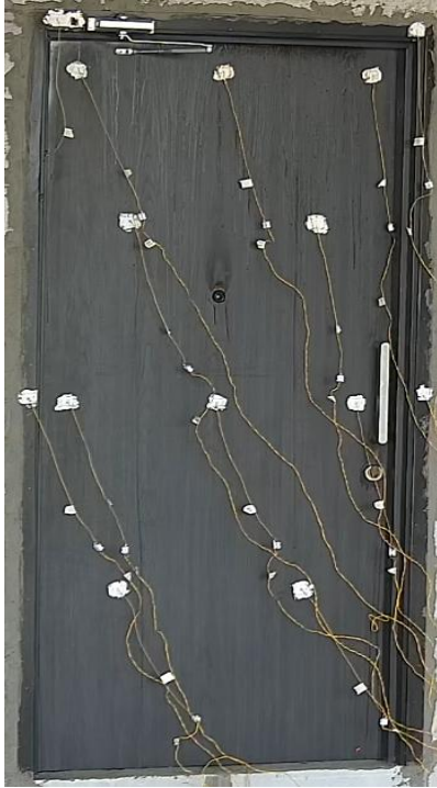
g) t = 75 min, blackening was observed near the door viewer.
