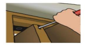
The bottom pivot bracket can be easily adjusted by loosening the lock nut and screwing the pivot in or out to adjust the height, you need to adjust it to achieve a gap of 3mm between the top of the door and the frame when the door is installed. A hole in the floor under the bracket will be needed to allow the bolt to be screwed downwards (remember to tighten the lock nut back up when adjustments are complete). Please check for under floor pipes and/or other services prior to drilling.
